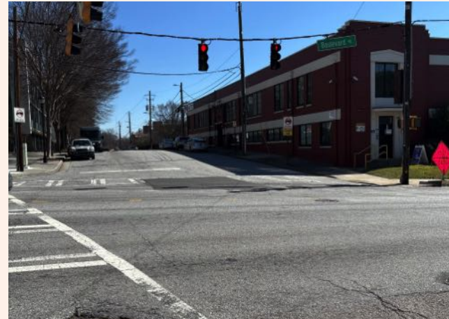
8 Skewed intersection allows vehicles to make turns at high speeds; pedestrian crossing is long and exposed.
