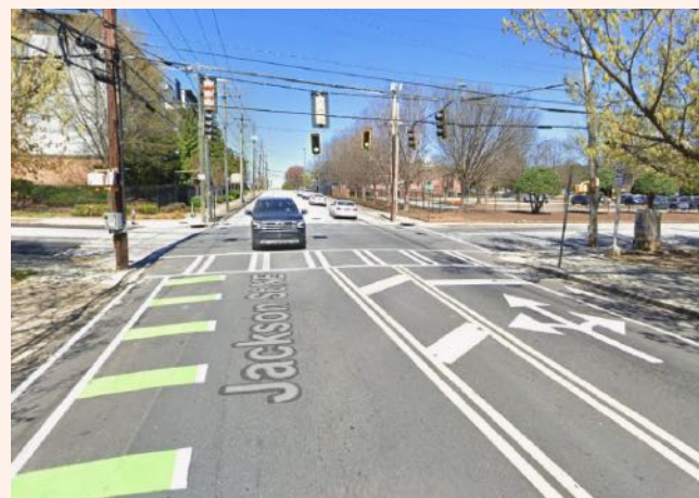
13 Drivers park on sidewalks near intersection. School zone flashing beacons and signage are not highly visible to drivers (eastbound). Removal of left turn lane for bike lane has created issues with vehicle queuing and congestion.
