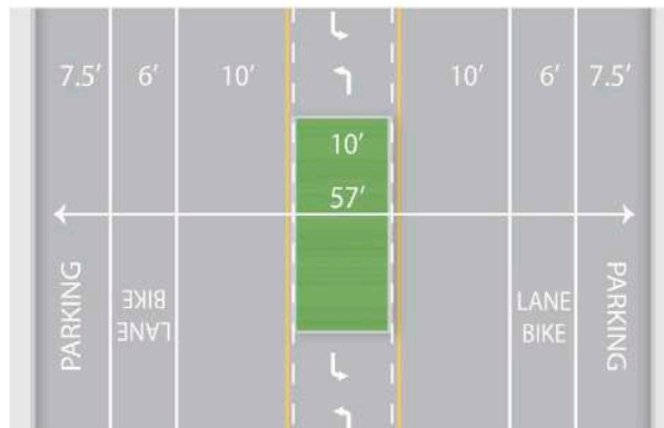
Collector with medians interspersed with turn lanes
