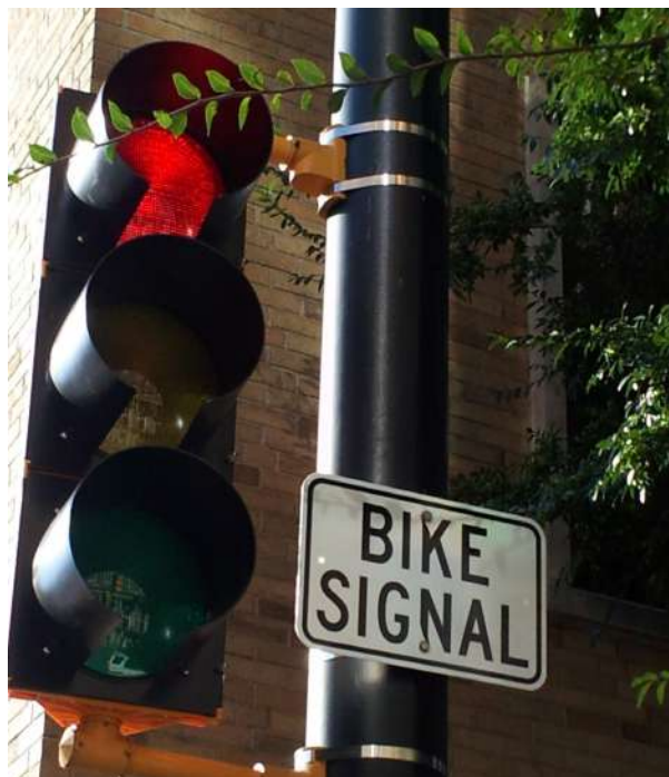
A leading bicycle interval is used at the intersection of W Peachtree St and 5th St to give westbound bicyclists a head start before left-turning motorists.
