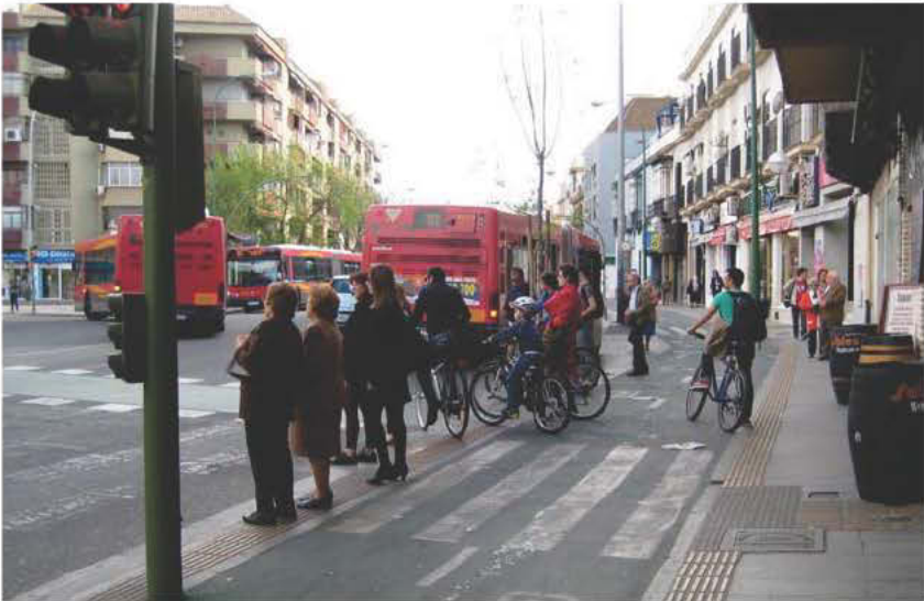
The raised cycle track approach to 10th Street along Williams will function similarly to the one above. It is designed to provide vertical separation from motor vehicles. It also provides space for pedestrians and bicyclists to wait before crossing Williams Street to the 10th Street bridge.
