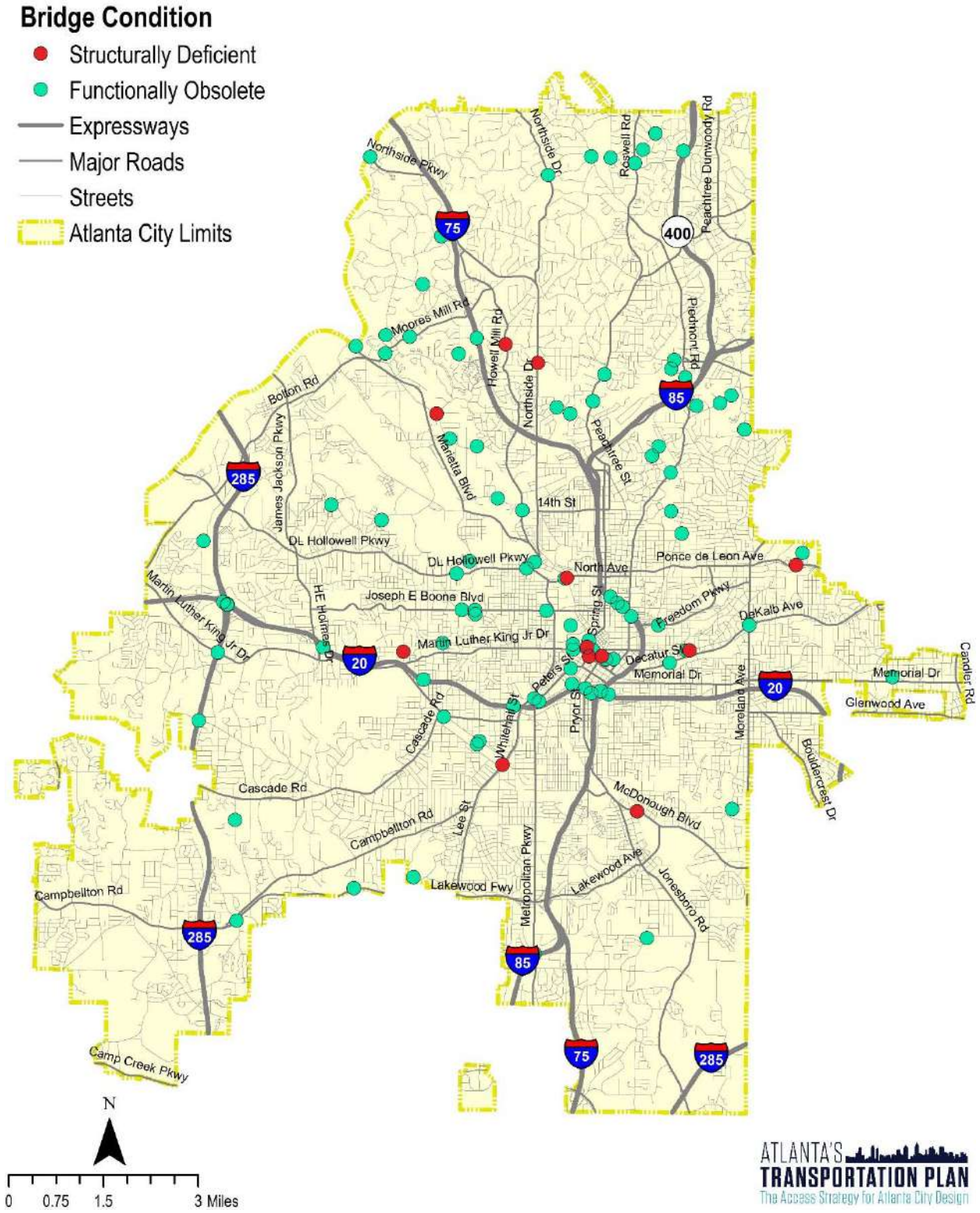
FIGURE 5: EXISTING BRIDGE CONDITIONS (2017)
